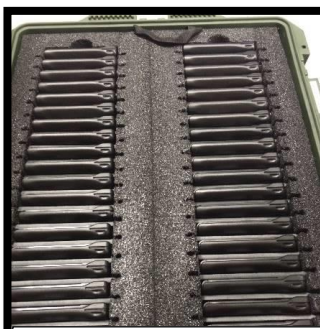
Case specially designed and cut for radio batteries. Terminals reversed to prevent contact.
