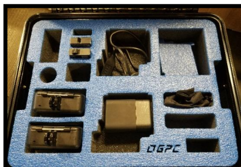
Pelican case with foam cut to shape for radios, batteries and charger. Batteries wrapped and surrounded by foam.
