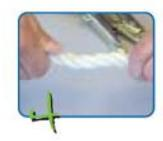
4) Rope Lanyard – Rotate the rope lanyard while inspecting from end-to-end for any fuzzy, worn, broken or cut fibers. Weakened areas from extreme loads will appear as a noticeable change in original diameter. The rope diameter should be uniform throughout, following a short break-in period.
